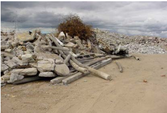
Stockpiles of concrete at various stages of pre-processing at Ward Resource Recovery, Auckland
