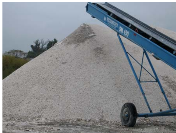
Ground and recycled gypsum without paper, Crusaders Landscaping, Christchurch
